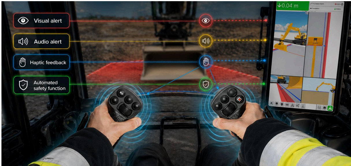
Concept illustration: haptic feedback in the A9 joystick grip can add a tactile communication layer to machine-control information.
